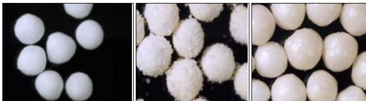
FIGURE 1: EMPIRICAL FORMULATION PROCEDURE OF LANSOPRAZOLE DR 15 MG CAPSULES: (A) SUGAR SPHERES, (B) DRUG LAYERED PELLETS, AND (C) ENTERIC COATED PELLETS 14
