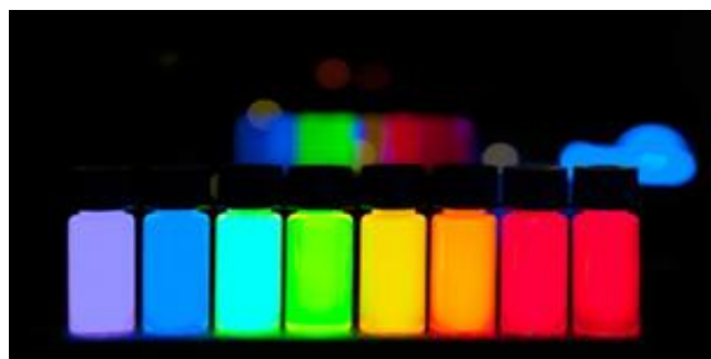
FIG. 1: QUANTUM DOTS WITH GRADUALLY STEPPING EMISSION FROM VIOLET TO DEEP RED ARE BEING PRODUCED IN A KG SCALE AT PLASMA CHEM DMBH 8
