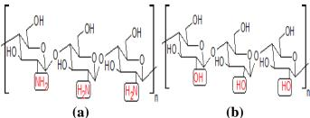
FIG.2 SHOWING STRUCTURES OF (a) CHITOSAN AND (b) CELLULOSE
