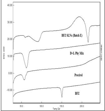
FIG. 3: DSC SCANS FOR BFZ, PRECIROL, D+L PHY MIX (DRUG + LIPID PHYSICAL MIXTURE) AND BFZ SLNS (BATCH E)
