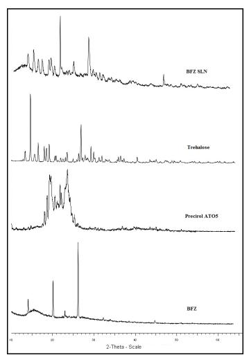
FIG. 2: XRD PATTERNS FOR BFZ, PRECIROL ATO5, TREHALOSE AND BFZ SLNs
