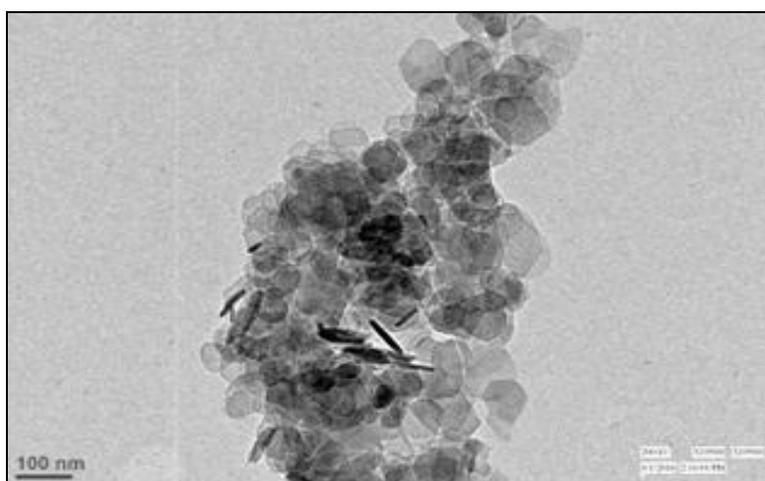
FIG. 7: TEM IMAGE OF MGO NANOPARTICLES (100 nm)
