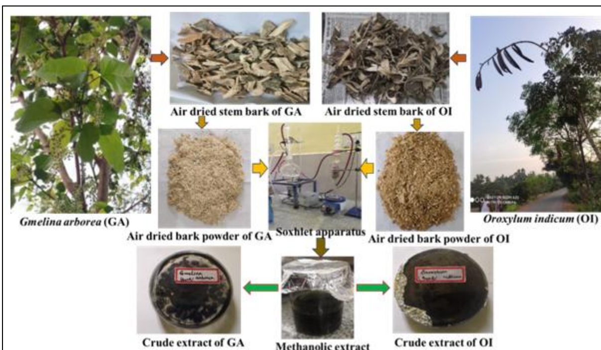
FIG. 1: PREPARATION OF METHANOLIC CRUDE EXTRACT OF Gmelina arborea AND Oroxyllum indicum STEM BARK
