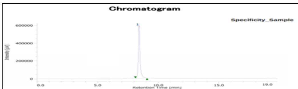
FIG. 1: SPECIFICITY PEAK PURITY CHROMATOGRAM OF (S)-(-)-AMLODIPINE-O, O-DI-P-TOLUOYL-D-TARTRATE
