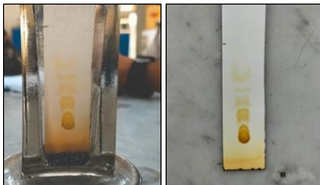
FIG. 7: TLC PROFILE OF SWERTIA CHIRAYITA PLANT EXTRACT UNDER UV LIGHT (366 NM) SHOWING SEPARATION OF PHYTOCONSTITUENTS USING DIFFERENT SOLVENT SYSTEMS. DISTINCT BANDS WITH VARYING Rf VALUES INDICATE THE PRESENCE OF COMPOUNDS WITH DIFFERENT POLARITIES
