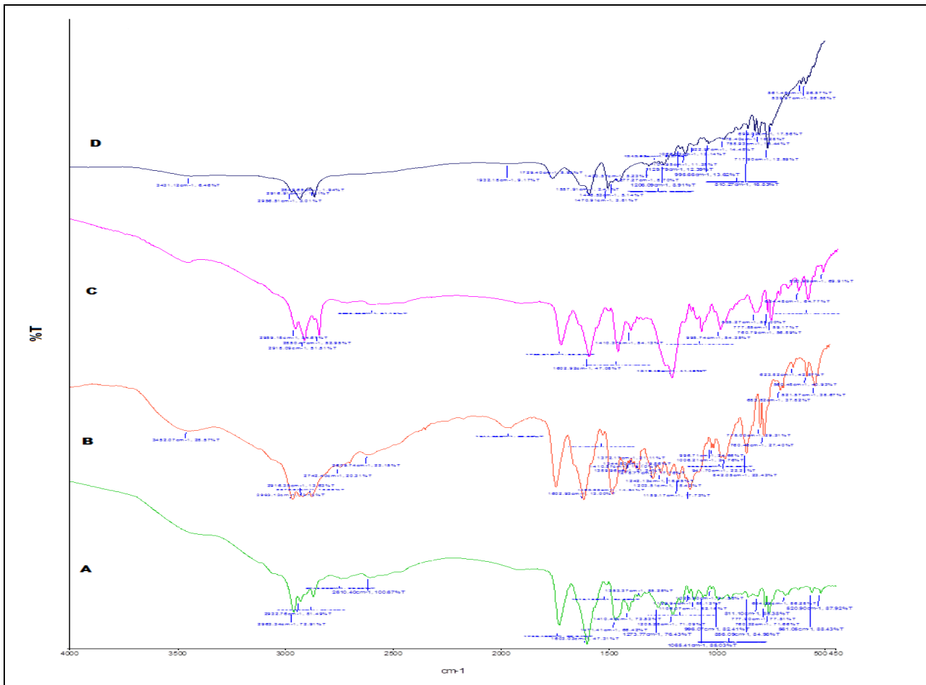
FIG. 2: COMPATIBILITY STUDY OF DRUG AND EXCIPIENT BY FTIR (A) VALSARTAN (B) VALSARTAN + POLOXAMER 188 (C) VALSARTAN + SODIUM STEARATE (D) VALSARTAN + SODIUM LAURYL SULFATE
