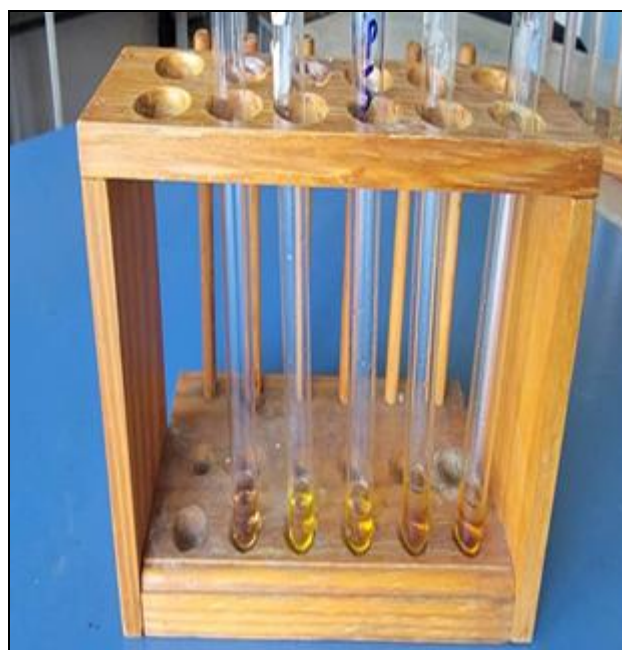
FIG. 2: DPPH RADICAL SCAVENGING ASSAY SET-UP SHOWING THE COLOUR GRADIENT (PURPLE TO PALE YELLOW) OF THE REACTION MIXTURE ACROSS DECREASING EXTRACT CONCENTRATIONS, REFLECTING INCREASING RADICAL-SCAVENGING ACTIVITY
