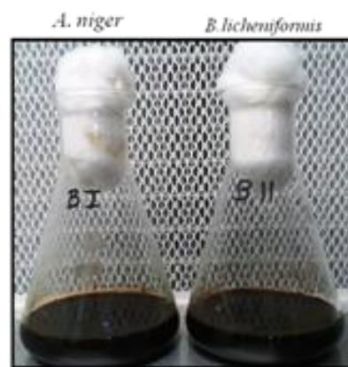
FIG. 14: SUPERNATANT (CRUDE ENZYME) COLLECTED AFTER CENTRIFUGATION OF FERMENTED BANANA PEEL WASTES BY WILD TYPE MICROORGANISMS
