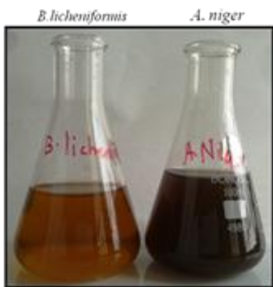
FIG. 15: SUPERNATANT (CRUDE ENZYME) COLLECTED AFTER CENTRIFUGATION OF FERMENTED POTATO PEEL WASTES BY WILD TYPE MICROORGANISMS
