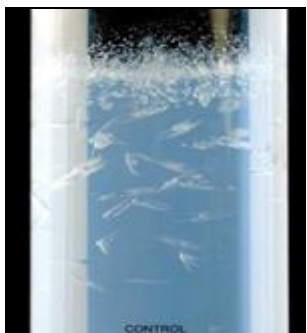
PLATE 1: CALCIUM HYDROGEN PHOSPHATE DIHYDRATE CRYSTALS IN SODIUM-META SILICATE GEL
