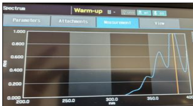
FIG. 2: UV SCAN OF THE STANDARD SOLUTION OF AMPHOTERICIN B
