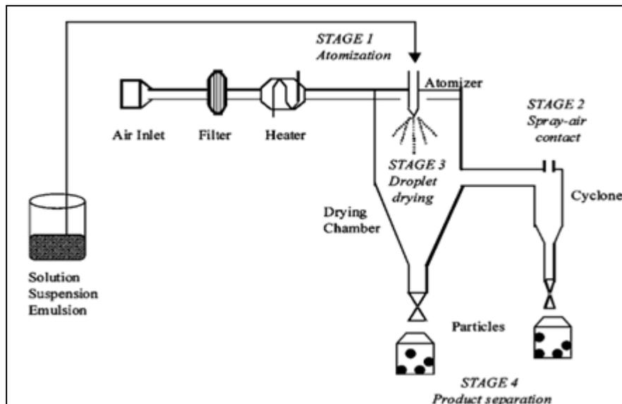
FIG. 1: SCHEMATIC DIAGRAM OF SPRAY DRYER; (ADAPTED FROM PATEL TEJAS ET AL., 2012)
