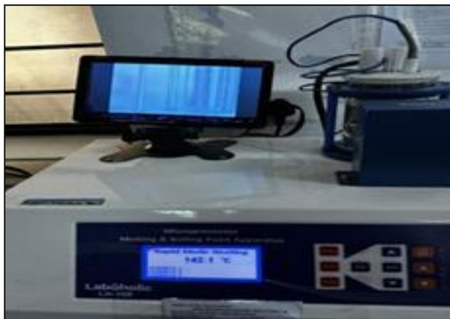
**FIG. 1: MELTING POINT OF CLINDAMYCIN PHOSPHATE**
