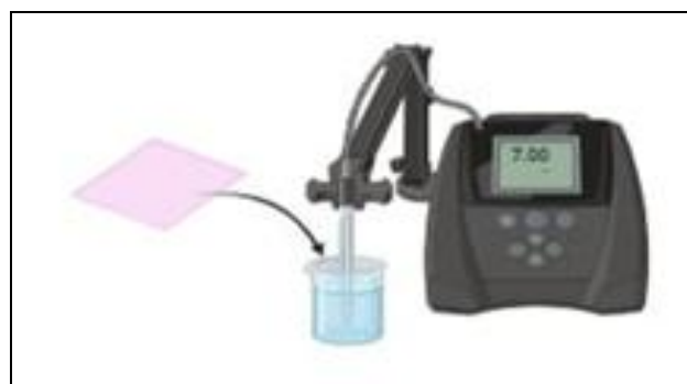
FIG. 6: MEASUREMENT OF SURFACE pH
