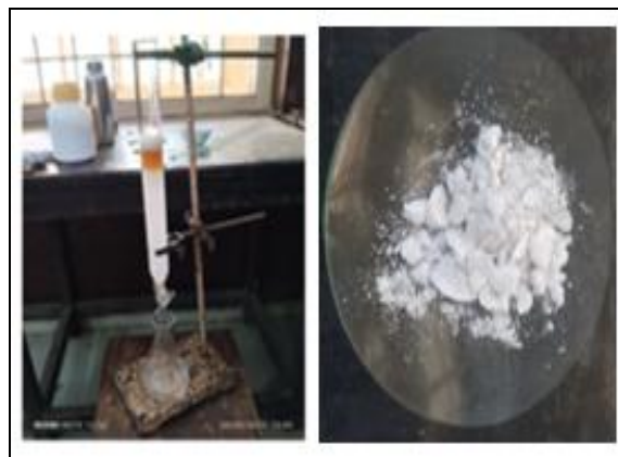
FIG. 2: COLUMN CHROMATOGRAPHY FOR PURIFICATION AND PURIFIED TETRABENZOYL ELLAGIC ACID
