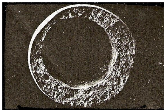
Fig 2: Scanning Electron microscope (SEM) of microballoons cross section
