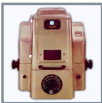
FIG. 1: INFRARED MOISTURE BALANCE
