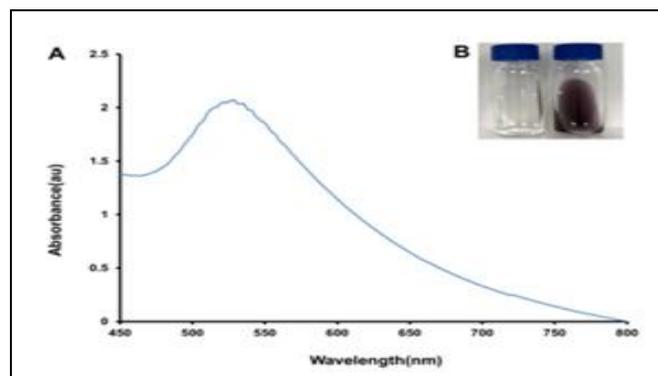
FIG. 1: A, UV-VISIBLE ABSORPTION SPECTRUM OF OKRA-AuNPs; B, COLOR CHANGES IN THE REDUCTION REACTION OF Au<sup>3+</sup> IONS
